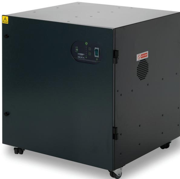
Bespoke fume extraction unit tailored to match the GCC C180 laser engraver. The dimensions of the unit allow the C180 to fit perfectly onto the extractor, effectively doubling it up as a work station. The unit is also offered with an onboard air compressor to provide the laser with its air assist requirements and comes complete with extraction hose kit and compressor link up on compressor models.
