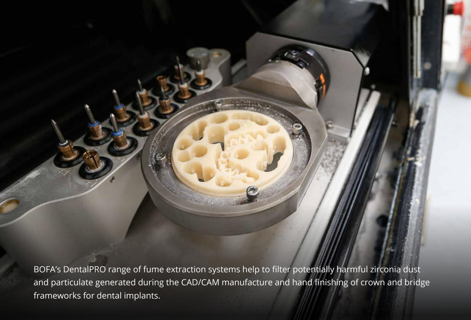
BOFA's DentalPRO range of fume extraction systems help to filter potentially harmful zirconia dust and particulate generated during the CAD/CAM manufacture and hand finishing of crown and bridge frameworks for dental implants.
