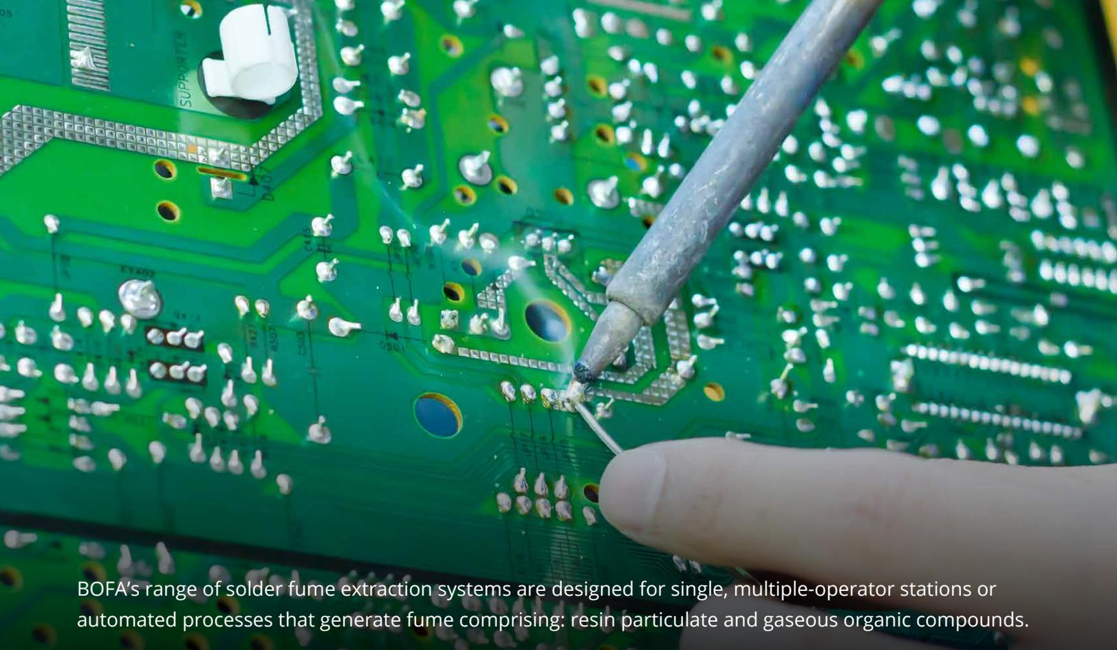
BOFA's range of solder fume extraction systems are designed for single, multiple-operator stations or automated processes that generate fume comprising: resin particulate and gaseous organic compounds. Our range comprises two types of systems: tip ('T') extraction for high pressure/low airflow soldering processes, and volume ('V') for low pressure/high airflow electronics processes.
